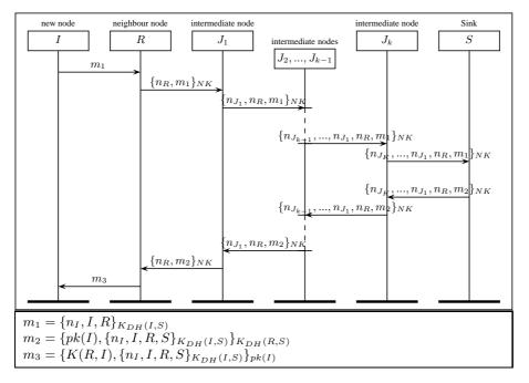
Fig. 3:  $IJS_{NK,dec/enc}$ : The intermediate nodes  $J_i$  decrypt, add a nonce value and encrypt the result message before forwarding it. It uses the network key to encrypt/decrypt this messages.
