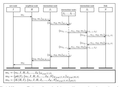
Fig. 4:  $IJS_{K,dec/enc}$ : The intermediate nodes  $J_i$  decrypt, add a nonce value and encrypt the result message before forwarding it. They use the session key to encrypt/decrypt this messages.
