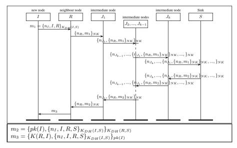
Fig. 5:  $IJS_{NK,onion}$ : The intermediate nodes  $J_i$  add a nonce and encrypt the request message and forward it to S.
