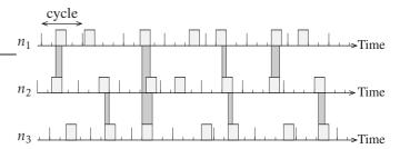
**Figure 1.** Example of the activities of three neighbor nodes with the protocol of [26], with a duty-cycle of 25% (this long duty-cycle is chosen for clarity).
