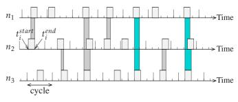
**Figure 2.** Example of the activities of three neighbor nodes with the SLACK-MAC protocol, with a duty-cycle of 25% (again, this long duty-cycle is chosen for clarity).
